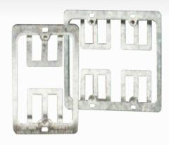
Mounting a flush mount wall plate without a back box is easy. Brackets insert into wall opening, flexible tabs bend up to secure the bracket to the opening. Standard screw holes accept all wall plate configurations.
